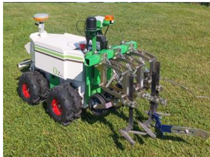
Weeding Relievre blade and goose foot point
