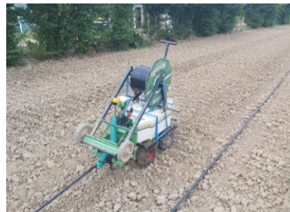
Unwinding drip Tape & wire
