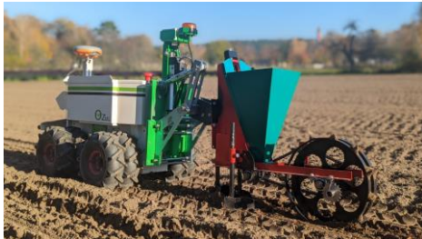
Seeding – Double Jang Automation & simple Ebra seeder
