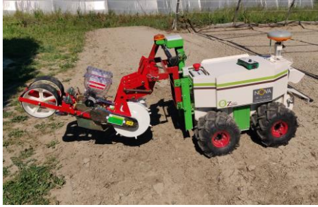
Seeding – Double Jang Automation & simple Ebra seeder
