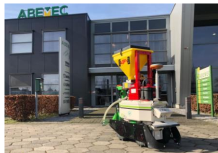
Band fertilizer spreader and broadcast Seeding
